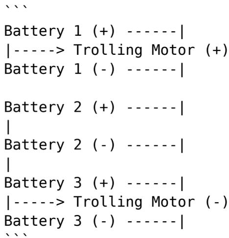
This diagram illustrates the series connection where the batteries are linked, providing a total of 36 volts to the trolling motor.
